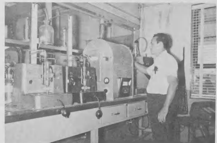
Senior Lab Assistant Francisco Marquez of the Inspection Lab determines % sulfur content of HDS products on Dietert machine. Sr. Lab Assistant Francisco Marquez di Inspeccion Lab ta determina % di azufre den productos di HDS ariba e machine Dietert.
